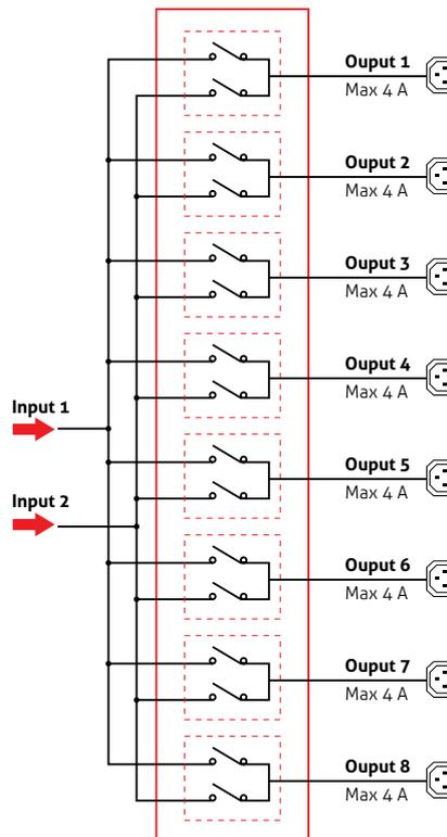
Multi Switch is a rackmount source transfer switch that can supply up to eight loads from two AC power sources. Should one source fail, the other automatically powers the load. The sources can be two separate AC sources including mains power and UPS, or a combination of the two.
